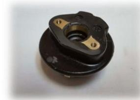
Rotor for the Bosch JF7 magneto.
