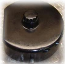
Magneto Cap for the Splitforf Dixie 800 fitted to the Hispano-Suiza V8 aero engine.
