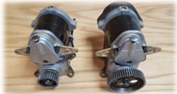
Pair of Bosch HL8 magnetos fitted to Curtiss JN-4D with Curtiss OXX6 aero engine.
