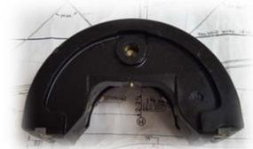
Magneto cap for the Bosch JF7 magneto.
