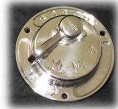
Chrome plated dual magneto switch with key for
