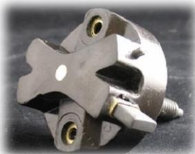
Rotor for the Splitforf Dixie 800 magneto fitted to the Hispano-Suiza V8 aero engine.
