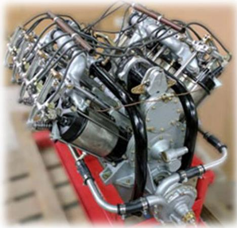
Curtiss OXX 6 engine rebuild fitted to a Curtiss JN-4D
