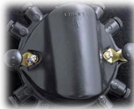
Liberty Distributor Cap Assembly complete with coil, condenser, rotor, and tension knobs. Fitted to Liberty V8.
